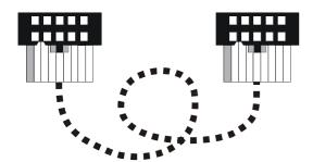
NA RYSUNKU POKAZANO WIDOK WTYCZEK OD GÓRY ORAZ ICH W Z A J E M N E U Ł O Ż E N I E W Z G L Ę D E M S I E B I E I ZAZNACZONEJ ŻYŁY TASIEMKI, PO PRAWIDŁOWYM WYKONANIU POŁACZENIA!!!
